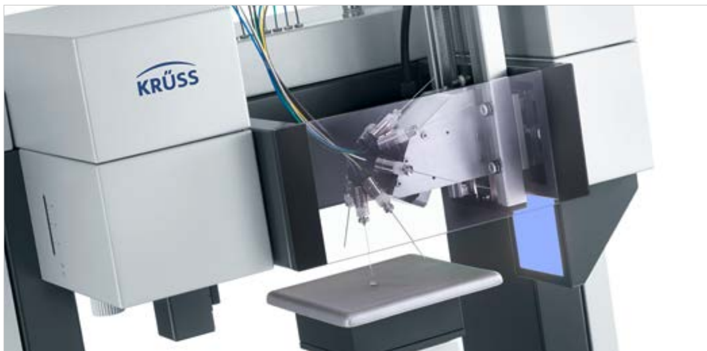
DSA100 with software-controlled multi-dosing system
