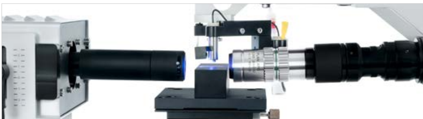
Dosing and analyzing picoliter drops with DSA30M
