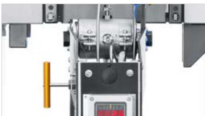
Sample positioning with closed pressure chamber
