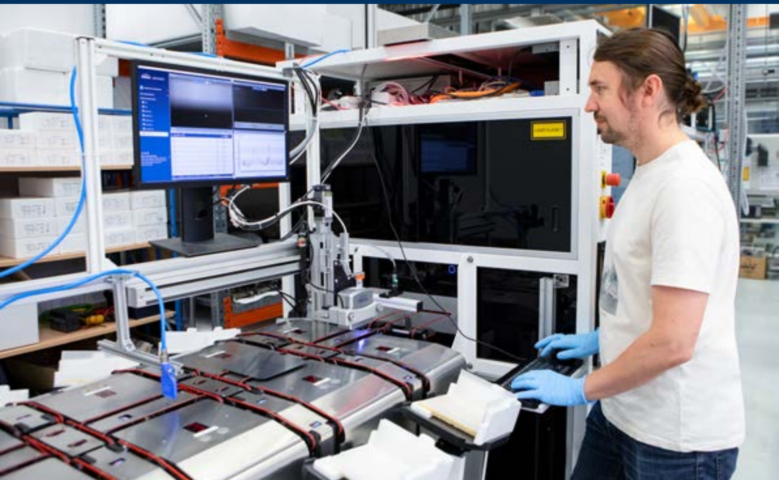
Ready for Industry 4.0: Inline cleanliness control with our MSA and ADVANCE at Fraunhofer CSP
