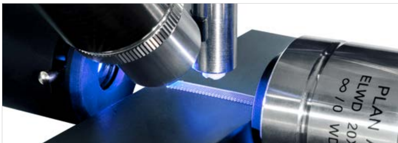
Dosing and analyzing picoliter drops with DSA100M
