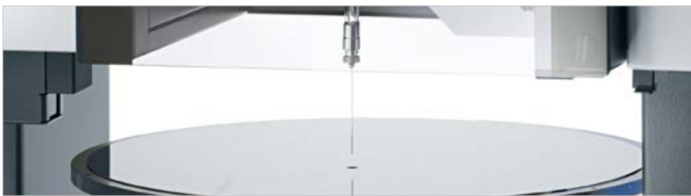
Fully automated drop positioning on a wafer
