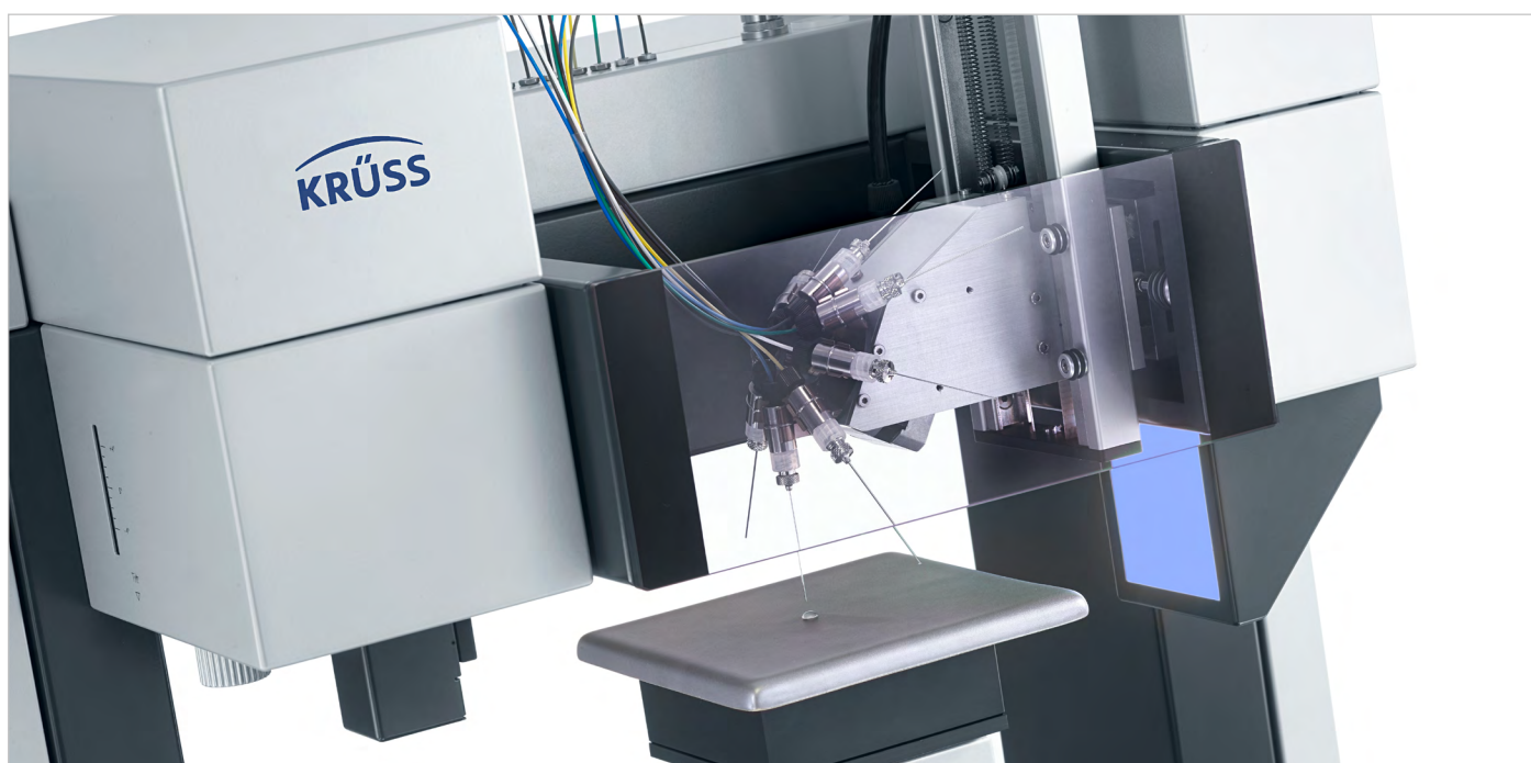
DSA100 with software-controlled multi-dosing system
