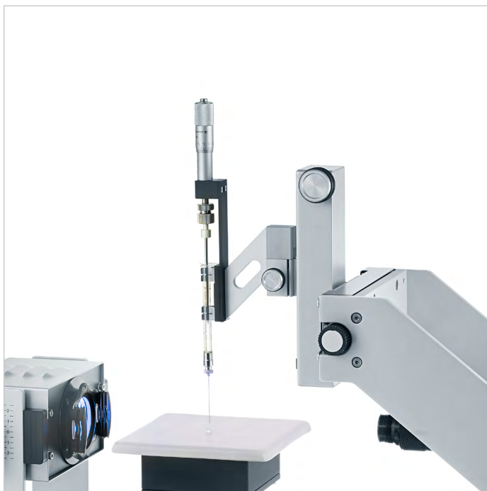
DSA30 with manual single syringe dosing unit
