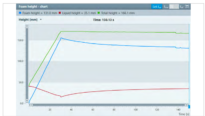
Simultaneous detection of total, foam, and liquid height
