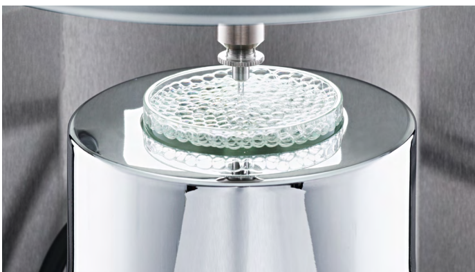
Sample stage with integrated temperature control
