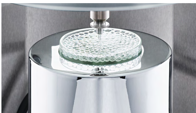
Sample stage with integrated temperature control
