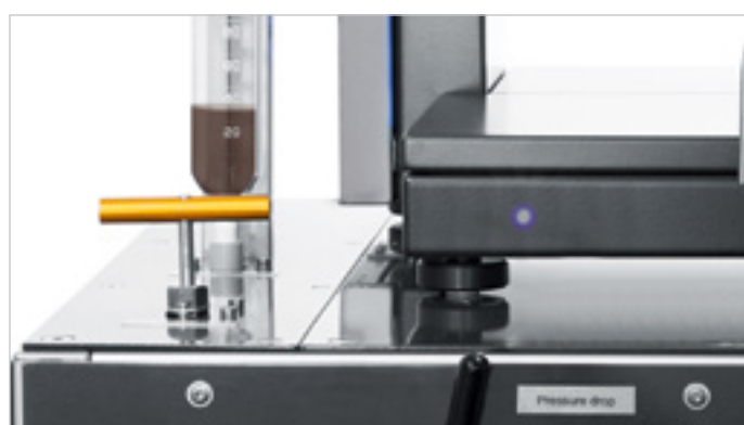
Either a gas or a liquid can be added as surrounding phase
