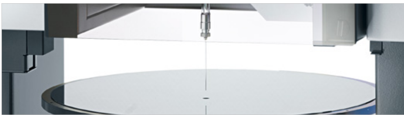
Fully automated drop positioning on a wafer
