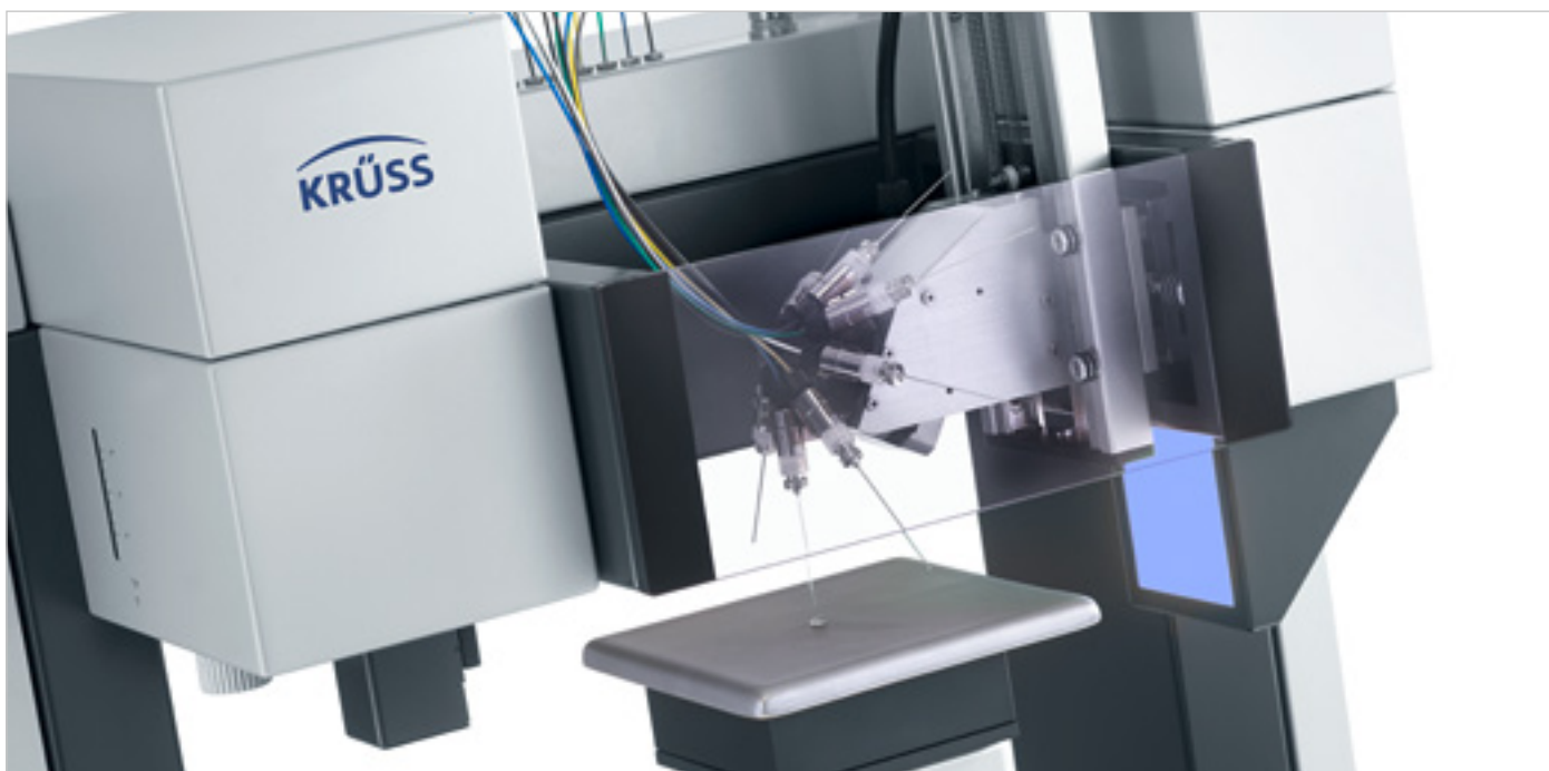
DSA100 with software-controlled multi-dosing system
