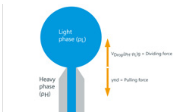
Measuring principle of a drop volume tensiometer
