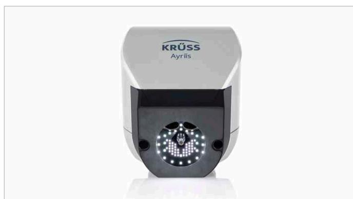
Hitech in a tight space: 90 LEDs generate reflection patterns for the three-dimensional reconstruction of the drop.
