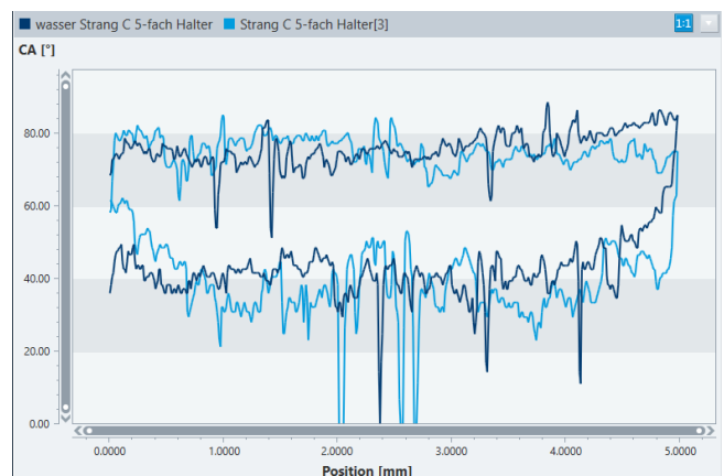
Fig. 2: Water contact angle vs. immersion depth as determined for five single fibers in parallel (double determination)
