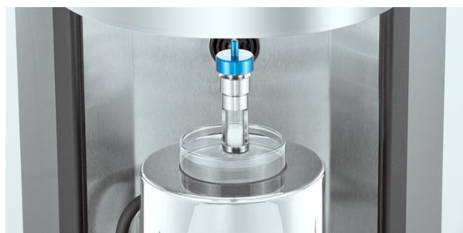
Fig. 4: The Washburn cell containing the compressed powder sample is attached to the force sensor
